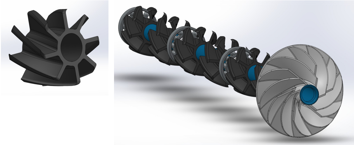
Figure 2. I6 engine turbines and compressor assembly. 105 mm compressor DIA. 730 mm OAL.
